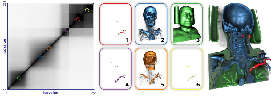
Figure 5: Representative isovalue selection algorithm applied to a CT data set. The isosurface similarity map is shown on the left and the six most representative isovalue are marked. The corresponding isosurfaces are depicted in the middle section numbered from one to six with decreasing relevance. The image on the right shows a cutaway view of the data set classified according to maximum similarity with the six isovalue.
