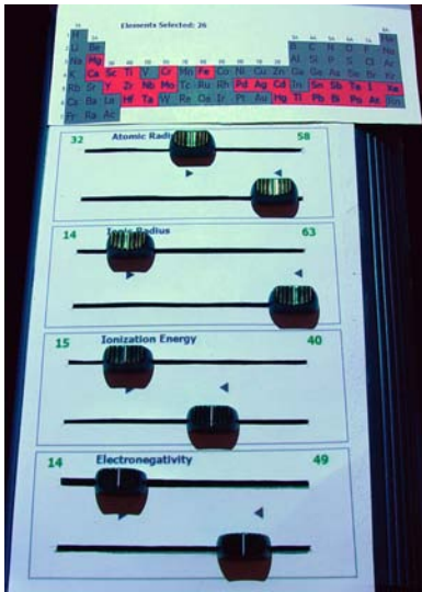
Figure 3: The physical interface for the periodic table. At the top the periodic table is projected, with currently selected elements in red. The sliders are below, with a projected overlay showing the controlled parameters and their current values. For example, the bottom two sliders have set the lower bound of electronegativity to 14 and its upper bound to 49.
