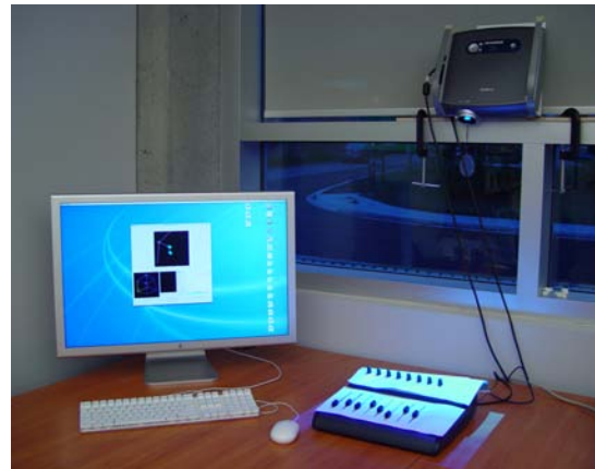
Figure 1: Physical setup: A Mac OS PowerPC with a 30-inch display, a Behringer BCF2000 mixing board, and a Canon Realis SX50 video projector. The parallel coordinates application is running, with the main window moved to the projector's display area.
