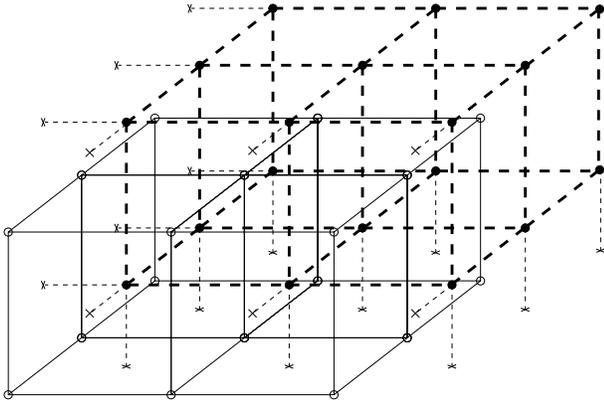
Figure 6: A bcc grid interpreted as two inter-penetrating Cartesian grids.
