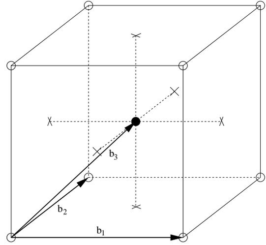
Figure 4: One cell of a bcc structure with base vectors  $b_i$ . The only difference to a simple cubic cell is one additional sample point right in the center of the cell, marked with a black dot.
