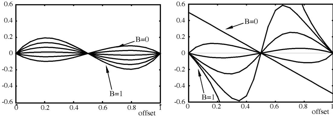
Fig. 6. Normalized error coefficients of the same filters that are shown in Fig. 4. (a) Errors for the cubic BC-spline interpolation filters and (b) errors for the cubic derivative filters. For our example, we chose  $B = C$  and varied  $B$  from 0 to 1 in steps of 0.2.
