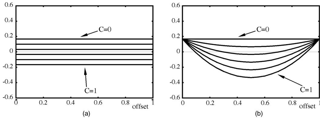
Fig. 8. Normalized error coefficients of the filters of Fig. 7. Errors for the (a) BC-spline interpolation filters and (b) BC-spline derivative filters are shown on the right. Because we applied the constrained  $2C + B = 1$ , these filters have better asymptotic error behavior (shown in Section 4.1.1 and Section 4.2.1). For our example, we varied  $C$  from 0 to 1 in steps of 0.2.
