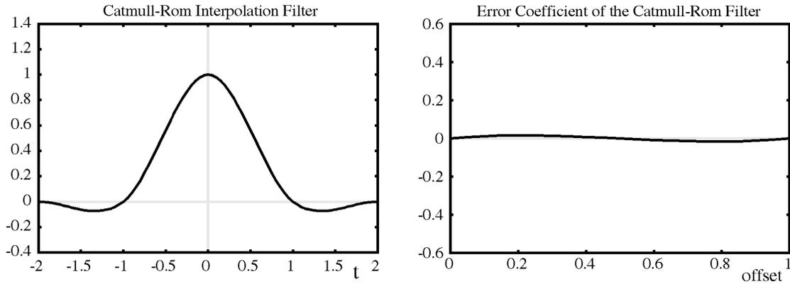
Fig. 5. (a) The optimal interpolation filter and (b) its error coefficient. We kept the scale of the  $y$  axis the same as for the other filters we have shown to better illustrate how the absolute errors compare.
