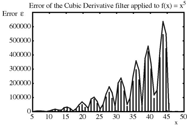
Fig. 3. The absolute error of the cubic derivative filter with the parameters  $B = 0$  and  $C = 1$  applied to a polynomial of fifth degree. We have also computed the error bound according to (9) using the result from Table 3 in Section 4.2. We can see that our error bound matches the actual error well. The actual error is shown as bars and the computed error-bound is drawn as a connected curve.
