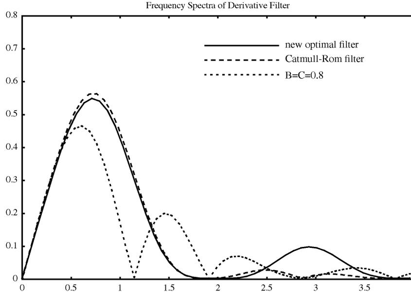
Fig. 10. Frequency plots of the derivative filters. The x and y axis are normalized by  $\pi$ . The straight line represents our new derivative filter. The dashed line represents the Catmull-Rom derivative filter ( $B = 0$  and  $C = 0.5$ ), and the dotted line represents a derivative filter for  $B = C = 0.8$ .
