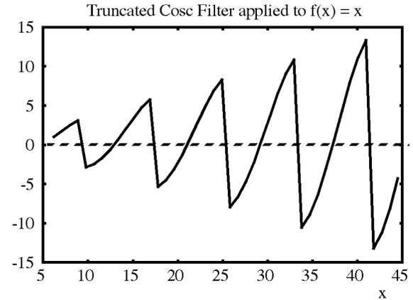
Fig. 2. Derivative reconstruction of the function  $f(x) = x$  using the truncated *Cosc* filter at  $M = 3$ . Since the coefficient  $a_0^w$  is not zero, we end up with artifacts that make the filter useless. (The expected result is the constant function  $f(x) = 1$ .)
