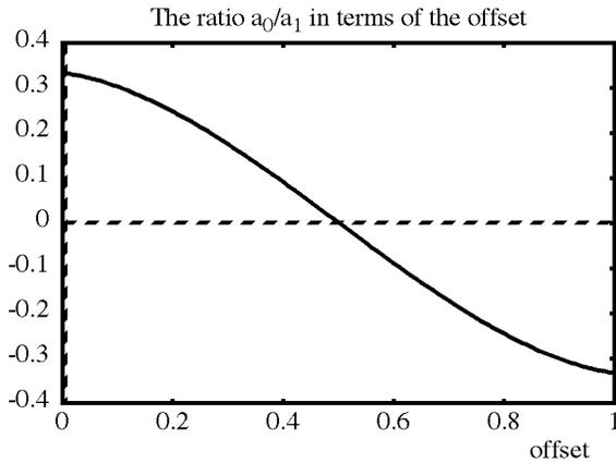
Fig. 1. The normalized coefficient  $a_0^w$  of the truncated *Cosc* filter in terms of the offset to the next sampled value. It is only zero for  $\tau = 0.5$ .
