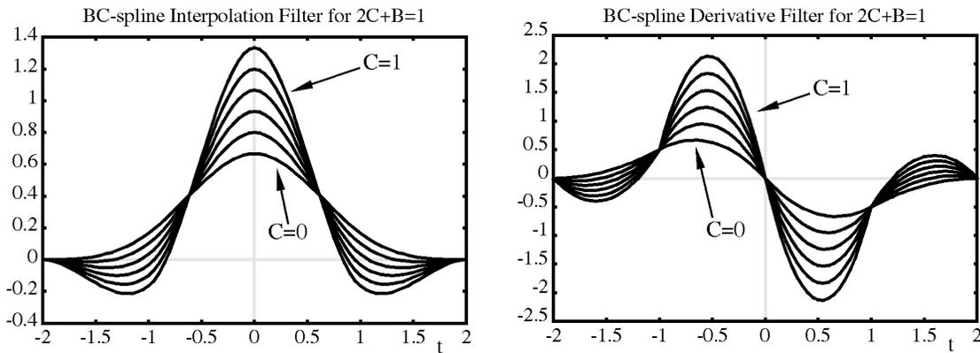
Fig. 7. Representatives of the class of (a) BC-spline interpolation filters and (b) BC-spline derivative filters with the condition  $2C + B = 1$ . Note these filters have a better error behavior than the general cubic splines. For our example, we varied  $C$  from 0 to 1 in steps of 0.2.
