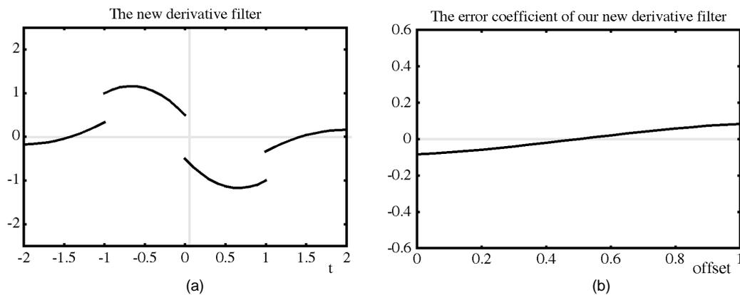
Fig. 9. (a) New optimal continuous derivative filter and (b) its error coefficient.
