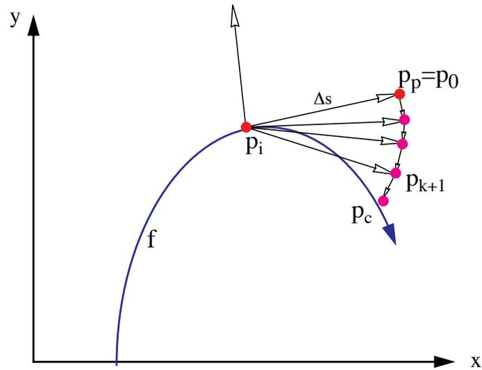
FIGURE 3. The corrector step. The Newton iterations and a forced circular movement of the iterates  $p_{k+1}$  converge towards an actual point on the curve  $p_c$ .
