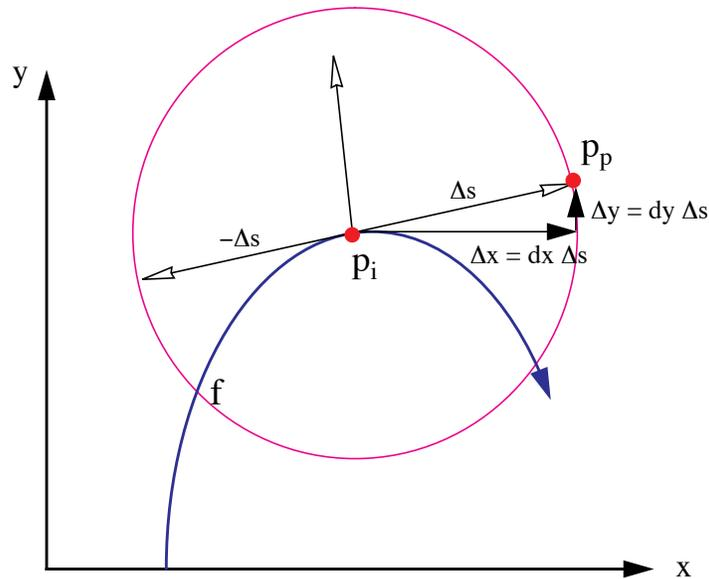
FIGURE 1. The predictor step. Here  $\Delta s$  is the step size we want to step along the curve starting at the initial point  $p_i$ . Because Equation (7) is only an approximation, the predicted value will not necessarily lie on the curve described by  $f$ .
