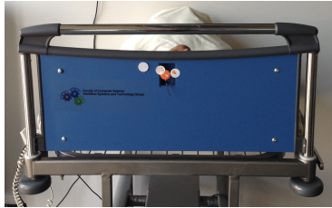
Fig. 2. NFC Reader Integrated into Resident's Bed
