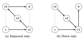
Fig. 1. A network update example, where forwarding paths have to be changed from the Surpassed (Fig. 1a) to the Down (Fig. 1b) state. Arrows represent paths on which traffic (e.g., from s to d) is forwarded, while (gray) undirected links between nodes represent unused links.
