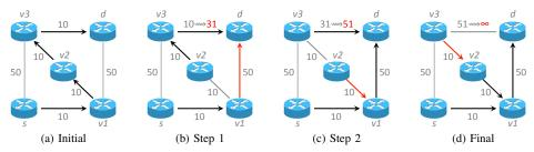
Fig. 3. Intermediate IGP weights that enable a loop-free reconfiguration for the example in Fig. 1.
