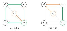
Fig. 13. In this network the task is to migrate consistently from the initial to the final state. If all flows and links have unit size, no consistent migration is possible: the destination has just incoming links of size two. If the flows just have a size of 2/3, one can migrate consistently in  $\lceil 1/(1/3) \rceil - 1 = 2$  updates by moving half of the flow size of 1/3 each time in parallel.
