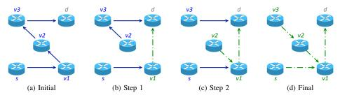
Fig. 5. Ships-in-the-Night reconfiguration that mimics the progressive link reweighting shown in Fig. 3. In each figure, the colors of router names indicate their respective control-plane preferences at the represented reconfiguration step.
