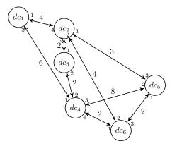
**Figure 2** Example topology: excerpt of Google B4 [16] (U.S. data centers only). Nodes here represent data centers (resp. OpenFlow switches located at the end of the corresponding long-haul fibers). Links are annotated with weights, and nodes are interconnected via ports (*small numbers*).
