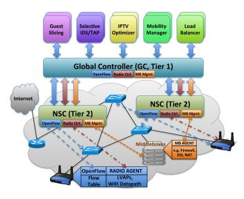
Figure 1: AeroFlux: NSCs are deployed close to the APs.
