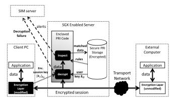
Figure 2. The PRI system inpects user session using the key sent by the agent. Matches are saved in a secured storage and alerts are sent to the corporate SIM server about detected anomalies.
