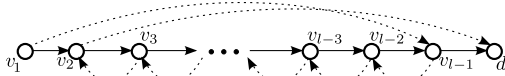
Figure 1: Network with old (solid) and new (forwarding) rules which requires l - 2 \in \Omega(n) rounds to update consistently when enforcing loop freedom. For example, v_3 cannot update before v_2 , and so on.
