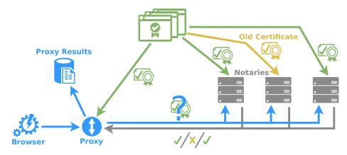
Fig. 2: Overview of our measurement setup.
