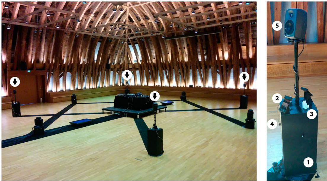
Figure 5. Left: The performance venue with the centre stage for the DJ and four marked stations. Right: A close up of one station with (1) its base, (2) mounted smartphones, (3) empty mounts, (4) pickup coils, and (5) a speaker as further described in the text.
