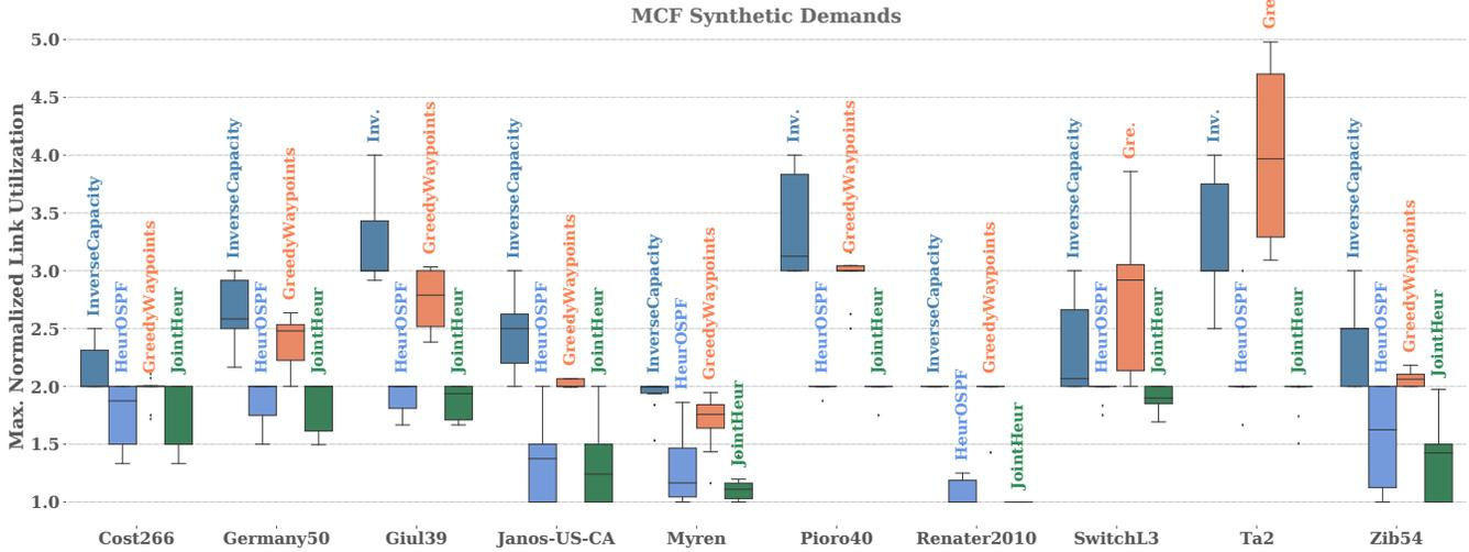
Figure 4: MLU statistics from different algorithms on the 10 largest capacitated non-tree topologies from TopologyZoo and SNDLib. Demands are generated using the MCF Synthetic method.
