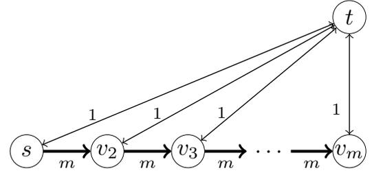
**Figure 1: See TE-Instance 1. There are  $m = n - 1$  unit-size demands from  $s$  to  $t$ . The optimal flow and JOINT are able to split one unit size flow away from the thick path at each node  $v_i$ . This is not possible under shortest path routing which causes a large gap in  $\Omega(n)$  between JOINT and LWO.**
