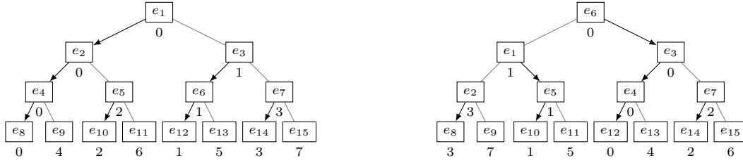
Fig. 1: Complete binary tree with rotor initial state of pointers (left) and after ROTOR-PUSH serves a request to element e_6 (right). Each node is represented by a rectangle and its label denotes the element stored at this node. Arrows represent states of rotor pointers. The number below a node denotes its flip rank: nodes with flip rank 0 constitute the global path. Serving element e_6 induces the following changes: Elements e_1 and e_2 are moved one level down along the global path, e_4 is moved to the initial position of e_6 , and e_6 is moved to the root. The states of rotor pointers of the two topmost nodes on the global path are flipped and the nodes' flip ranks are updated accordingly.
