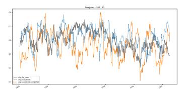
**Figure 5.** Plot depicting the time-varying DFA and Hurst exponents, using a 200-day input window and a 10-day step size between windows, close up for the years 1960–1980.
