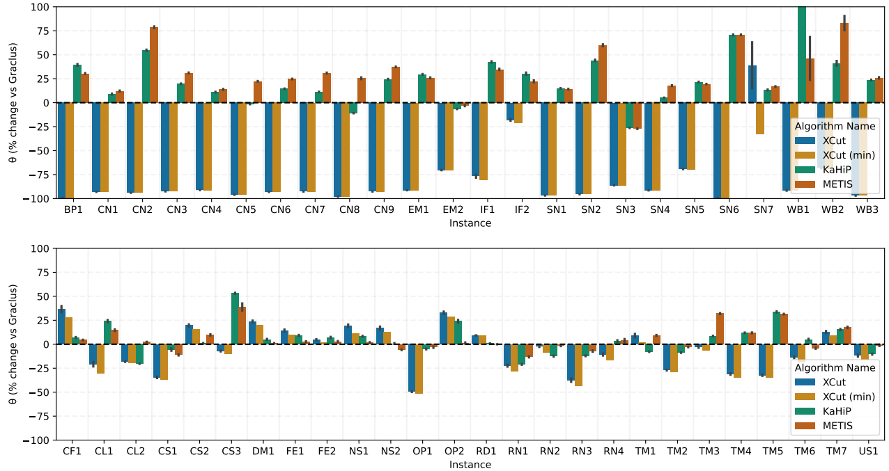
Figure 5: Percentage deviation of the returned normalized cut value relative to Graclus for k = 32 . This means that a value of -75\% indicates that the normalized cut value is 75\% lower (i.e., better). The thin black bars indicate the standard error across our runs. The top graph shows the disconnected IMDB graph (BP1), citation network instances (CN), email networks (EM), infrastructure graphs (IF), social networks (SN), and web graphs (WB), while the bottom shows the remaining instances. See the full version of the paper for details.
