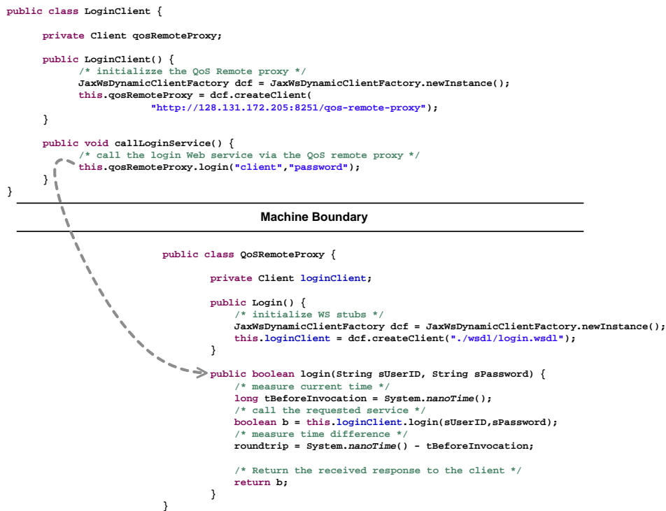
Figure 11: Measuring the round-trip time following the QOS REMOTE PROXY pattern
