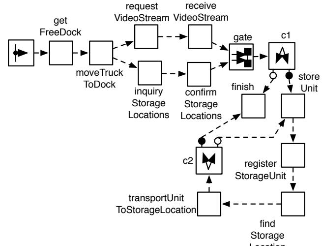
Figure 4. The DERA snapshot of the warehouse operator
