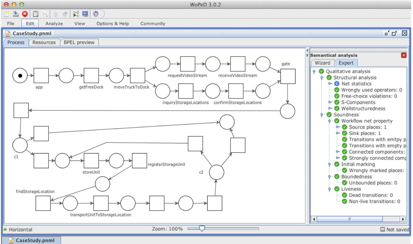
Figure 6. Petri nets-based analysis of a snapshot of the warehouse operator
