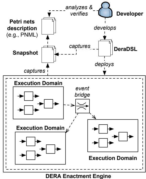
Figure 3. DERA development tool chain and system architecture
