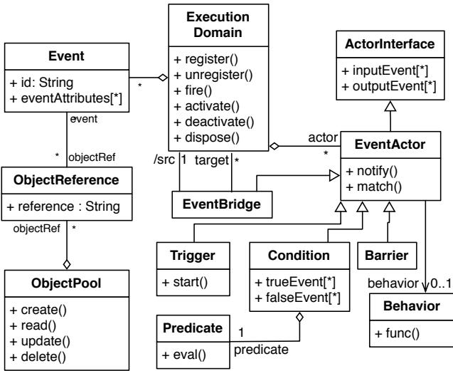
Figure 2. Meta-model for the primitive DERA concepts and their relationships [6]
