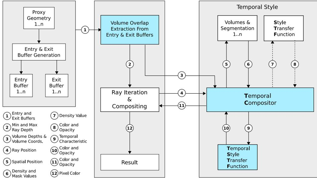
**Figure 2. Schematic overview of the TSTF based multi-volume raycaster. Blue indicates our extensions to the standard raycaster.  $n$  is the number of volumes. The encircled numbers indicate the processing order. The dashed lines are an optional part of the pipeline.**
