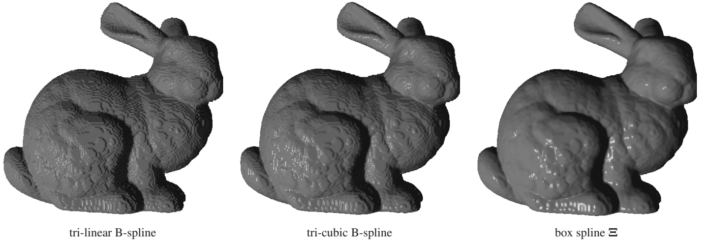
Fig. 10. The Stanford Bunny dataset voxelized with an 18 connectivity neighborhood at the sampling resolution of 182 \times 182 \times 182 .
