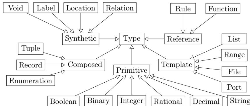
Figure 3.4: CASM-IR Type System (Inheritance Tree)
