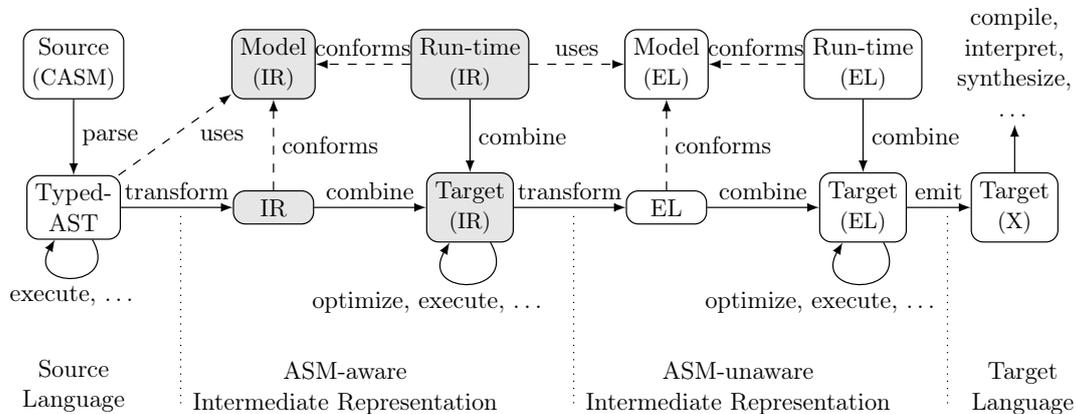
Figure 3.3: CASM System Design (High-Level Overview)
